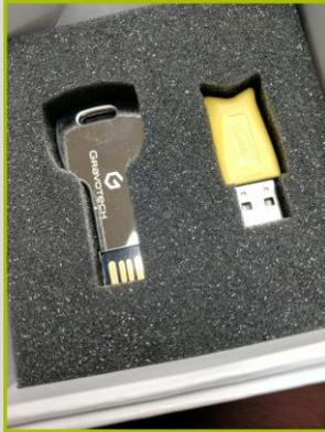
**Yellow Software Key (Dongle)** - Plugged in to USB port at all times to run 3DESIGN. Red light indicates the dongle is on.
